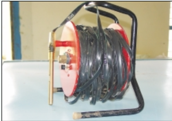
Ground water level measuring device
