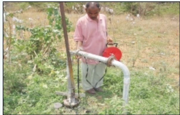
Farmers measuring level of ground water through measuring device
